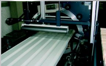
Automatic packaging for roof panels
