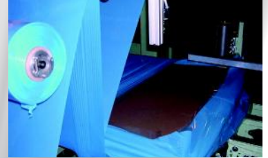
Multi layer wrapping with different materials.
