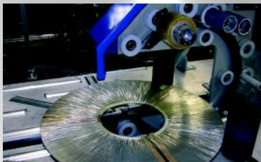
Horizontal wrapping machines for slitted coils. Semi- and fully automatic solutions for a weight up to 10t
